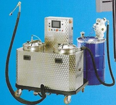
Dosing, mixing and dispensing unit
