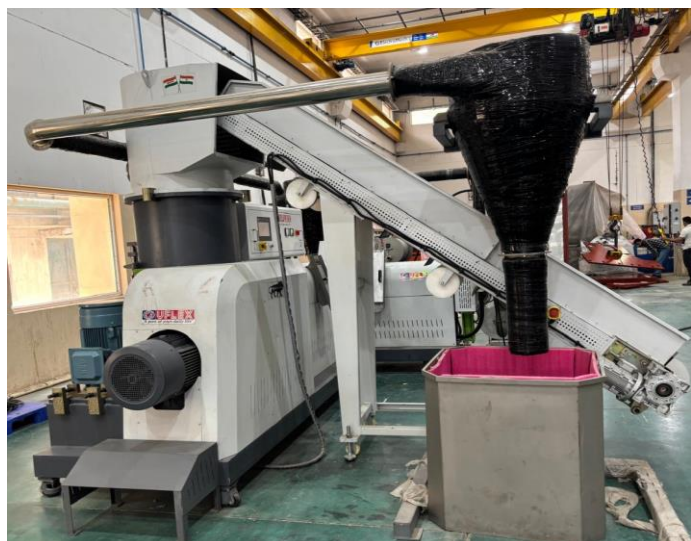
Live in action: UFlex's ReLAM 50 — a compact recycling unit transforming mixed flexible waste into reusable materials
