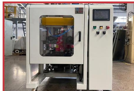
completely servo driven with an operator friendly human interface. It facilitates efficient vacuum pulling, smooth-motion cross & vertical seal technology that delivers superior quality seal with high seal integrity. This machine runs at a speed of 120 PPM with a very low rate of on-line rejections on snack packaging applications. This is the first Indian continuous type VFFS machine running at this high speed with minimal rejection meeting the standards of any international machines.
