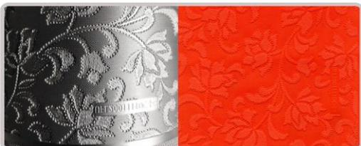
**b. Special Effects through Specialized Cylinders** - With the development of Laser Engraving specialized Cylinders that produces holographic and 2D effects, UFlex has achieved high depth tissue paper embossing and cotton handbag paper embossing, a feat never attempted before in the industry.
