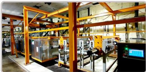
**a. Line Installation for Automated Chrome Plating on Rotogravure Cylinder** - The Cylinder Business of UFlex installed a new automated Chrome Plating Line for Rotogravure Cylinders that helps enhance efficiency and ensure consistency with improved print quality. It also launched Water-based Cylinders throwing up new opportunities for the business to tap into customers looking for green and cost effective printing processes.
