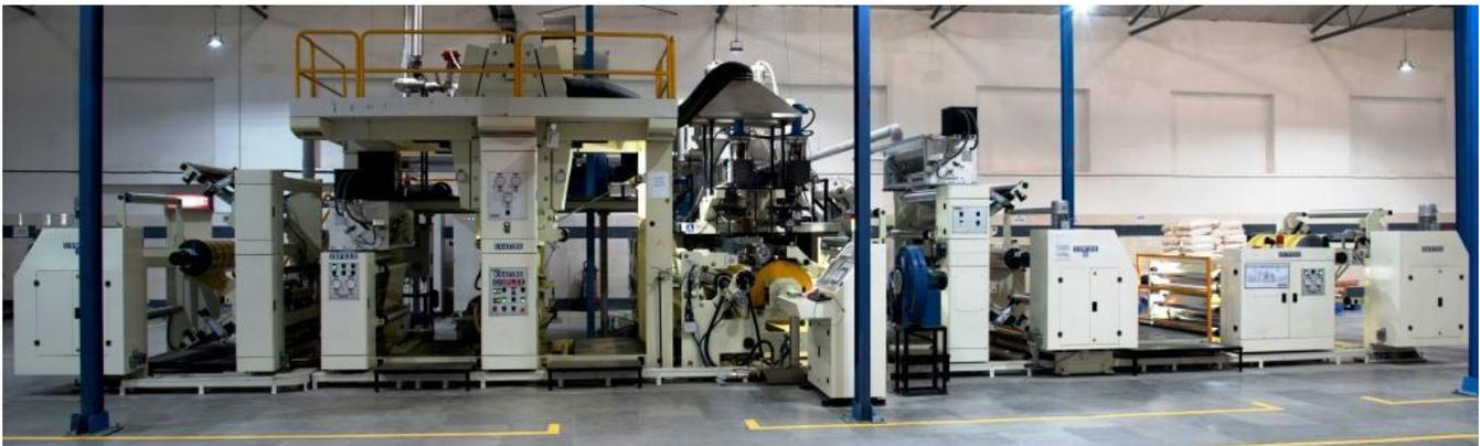
Second in line was its state-of-the-art **CI Flexo model 'Elisa'** designed for maximum operating speed of 400 mpm with high automation level in the form of sleeves and anilox removal system. Uflex is the first ever Indian company to make CI Flexo and its latest variant offers many value additions including an efficient Ink Washing system that helps in saving time as well as cost.
