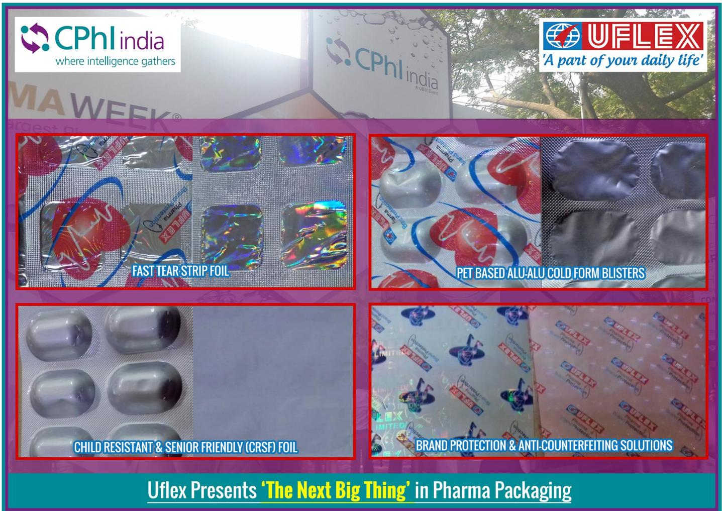
**Fast Tear Strip Foil:** Conventionally, Pharma companies have been using 30 and 40micron soft tempered Strip Foil pack laminate. Uflex has developed 20micron pin-hole free soft tempered foil. It contributes in providing higher yield gain of 36% leading to tremendous cost savings for Pharma companies. Offering excellent printing on matt finish with superior readability through multi-color reverse printing design on Special PET film in Special
