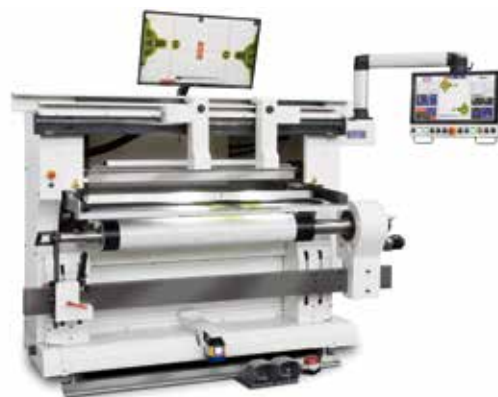
Automa 374, the latest generation and precise plate mounter made in Italy for the automatic centering of flexographic printing plates (patent pending) with microdots or crosses"
