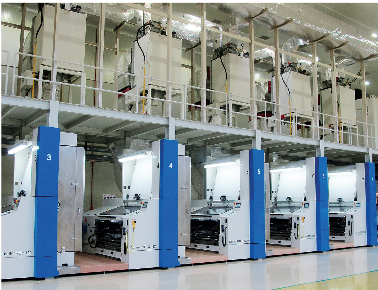
Gallus INTRO 1320 flexo press at the new Uflex Asepto plant in Sanand. Photo PSA
