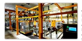
a. Line Installation for Automated Chrome Plating on Rotogravure Cylinder - The Cylinder Business of UFlex installed a new automated Chrome Plating Line for Rotogravure Cylinders that helps enhance efficiency and ensure consistency with improved print quality. It also launched Water-based Cylinders throwing opportunities for the business to tap into customers looking for green and cost effective printing processes.
