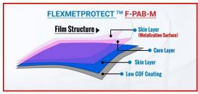
ultra-thin gauge high barrier specialty film markets. This includes the balloon film market and wherever low OTR and MVTR is needed, thus enabling balloon converters and end users to create dazzling, printable, metallized polyester inflatables that do not stress or snap and conserve seal property during the manufacturing process. F-PAB-M has an added 'Green' benefit due to the use of less material, giving
