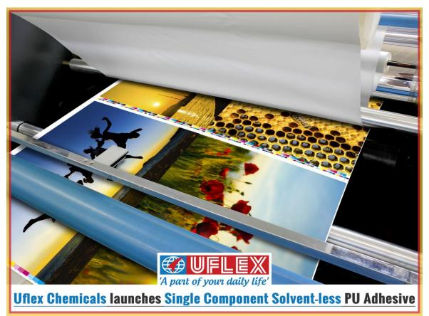
This moisture curing adhesive is designed for laminating film with printed and un-printed board or paper, with an average coating weight of 3 to 5 GSM (depending upon the thickness of the board).
