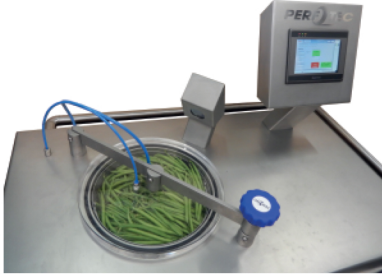
Step 1 Measure the respiration rate of the fresh produce with the Fast Respiration Meter
